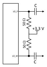
Figure 46. LO Port Operating In Output Mode Requires Load Resistors Or Inductors
