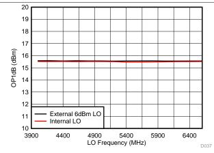
The LO frequency is capped at 6600MHz because IP1dB exceeds +10dBm when LO frequency goes beyond 6600MHz; The device can be damaged when input power is more than +10dBm.
