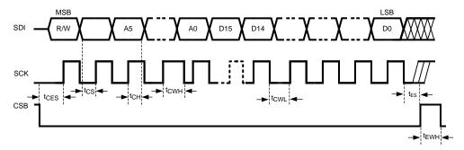
Figure 1. Serial Data Input Timing Diagram
