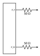
Figure 48. IF Interface Requires External Resistors for 1000hm Differential Matching
