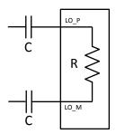
Figure 47. LO Port Operating In Input Mode
