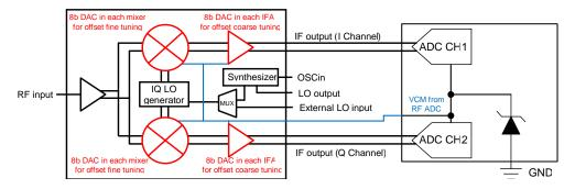
Figure 50. DC Offset Correction Diagram
