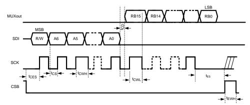
Figure 2. Serial Data Readback Timing Diagram
